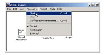
Simulink runs the simulation and plots the signal data in the Scope window.
